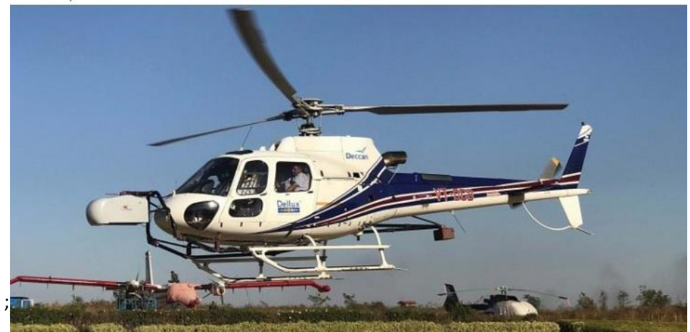
A helicopter equipped with Light Detection and Ranging system.
